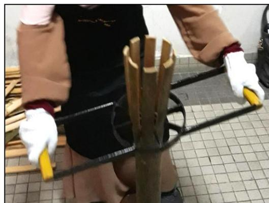
Figure 2: Cutting bamboo into long strips before extraction of fibres
