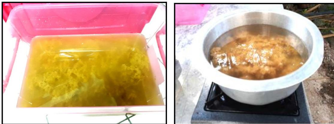
**Figure 4: Soaking of bamboo fibres before boiling (left) and boiling the fibres before beating (right)**
