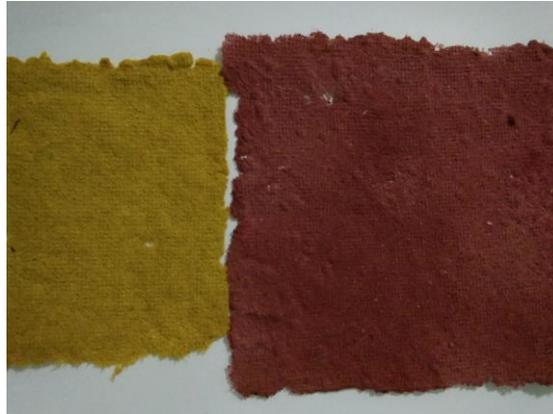
Figure 9: Bamboo paper samples show good absorbency of synthetic dyes
