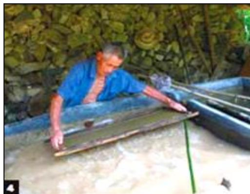
Figure 1: A villager dips a bamboo screen in and out of a vat filled with bamboo pulp to form sheets of paper on the screen.
