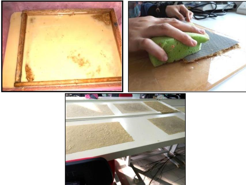
**Figure 5: Straining the pulp to form a sheet (A), using sponge to remove excess water from the sheet (B) and drying of the sheets on a flat surface**
