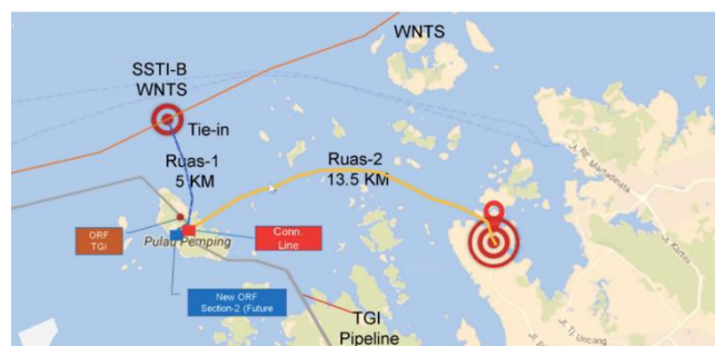
Fig. 2 Gas Pipelines System Pemping Island - Tanjung Uncang Batam
